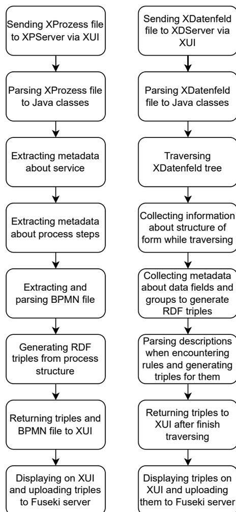
Figure 4: Workflow of the XPServer and XDServer.
